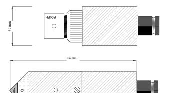
The UCP1A contact probe is a lightweight and versatile instrument that provides a means of carrying out underwater cathodic protection potential measurements.
