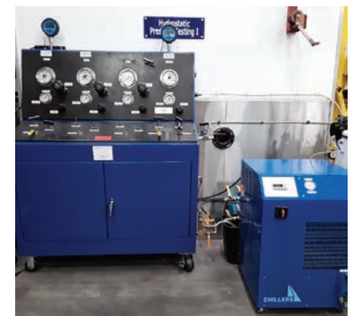
The pressure system controls located outside Hydrostatic Pressure Testing facility I (The chiller was not used for this test.)
