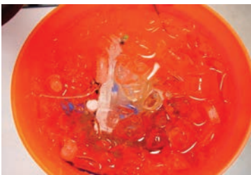
After over an hour at -55^{\circ}\text{C} , the connector is plunged into 0^{\circ}\text{C} ice water.
