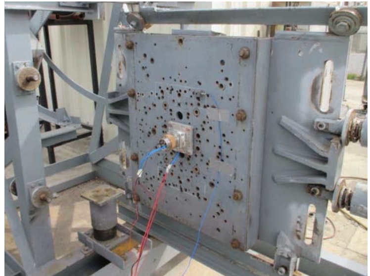
Operational signal transmission during shock testing of BIRNS connectors per MIL-S-901D Grade A Class I Type C, with impacts from the TOP/BACK (L) and SIDE (R).
