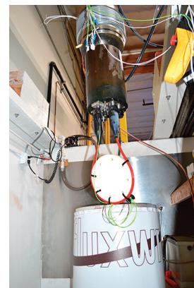
Low temperature/high pressure test capability simulates actual conditions at depth, with long-term continuous pressure testing in a controlled 2°C (±1°C) environment; programmable, automated multiple pressure cycles; real-time electrical and optical test data recording; and continuous digital output of pressure and temperature data.
