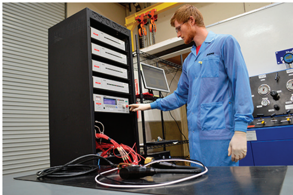
Final acceptance tests using a Kikusui TOS9213S DC DWV/IR Tester with high voltage scanners. This custom-made programmable system permits simultaneous testing of up to 16 electrical circuits at voltages up to 6kV, even while under hydrostatic pressure.
