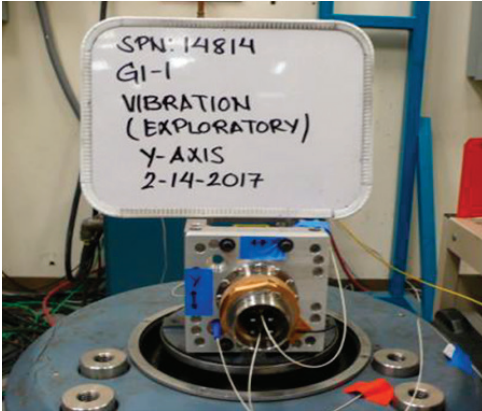
Exploratory, variable-frequency, and endurance vibrational testing performed per MIL-STD-167-1A, Type 1, Table III, to 14 Hz—no signal discontinuities before, after, or during vibration.
