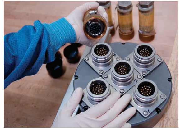
Preparing various inserts for high-pressure open-face hydrostatic testing.
