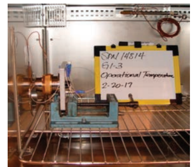
Inside the test chamber at +65^{\circ}\text{C} .
