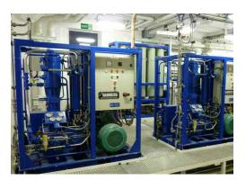
The Electric Gasmizer is the world's most popular gas reclaim system. Comprising simply of four main robust components, it is easy to see why. It will reclaim gas from two divers at down to 500msw/1,650fsw.
