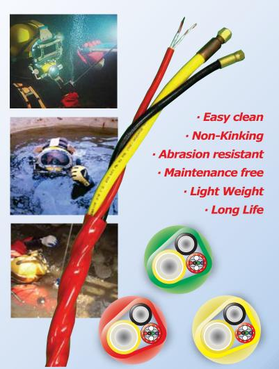
**Aquaflow SW** is the latest dive umbilical from the Diveline life-support product family. Based on the fully cabled 3 part Aquaflow "Classic" umbilical it features an extruded outer jacket of tough, abrasion resistant polyurethane. This jacket is specially made to conform exactly to the spiral shape of the "rope-like" construction beneath, this maximizes flexibility whilst providing unrivalled protection for the hose and cable components.
