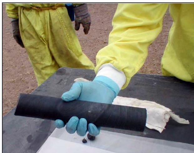
**Figure 7. LANL Radioactive Demonstration Vitrified Product Typical Core Sample**
