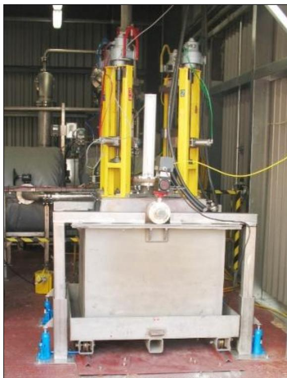
**Figure 3 - GeoMelt Demonstration System ICV Vessel**
