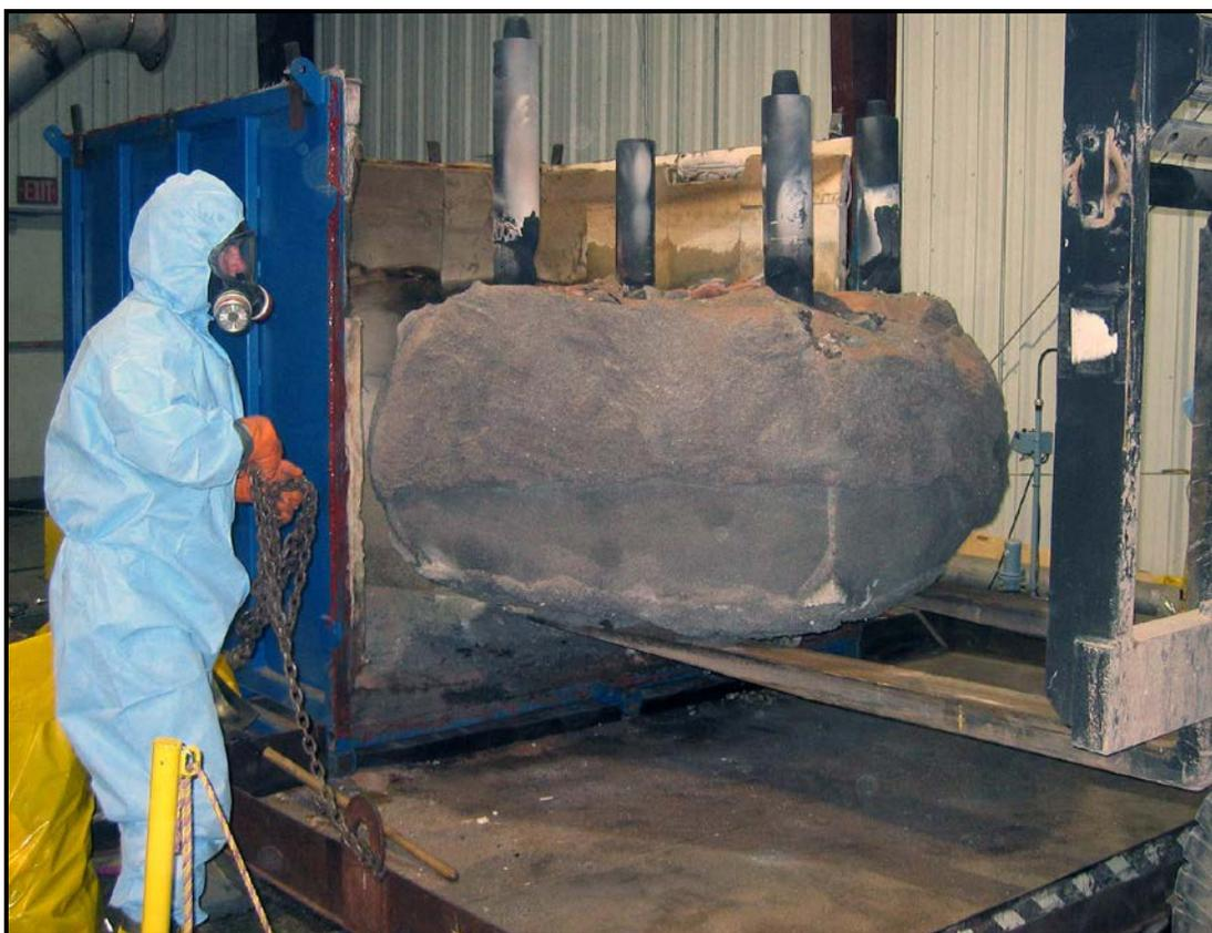
**Figure 5 - Removing vitrified product from the ICV™ Container. The exterior of the vitrified product is composed of high-temperature siliceous liner material that anneals to the block during melting. The block retains the symmetry of the container.**
