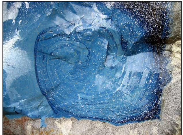
Figure 10. Flow Pattern in GeoMelt ICV Glass Indicates Mixing
