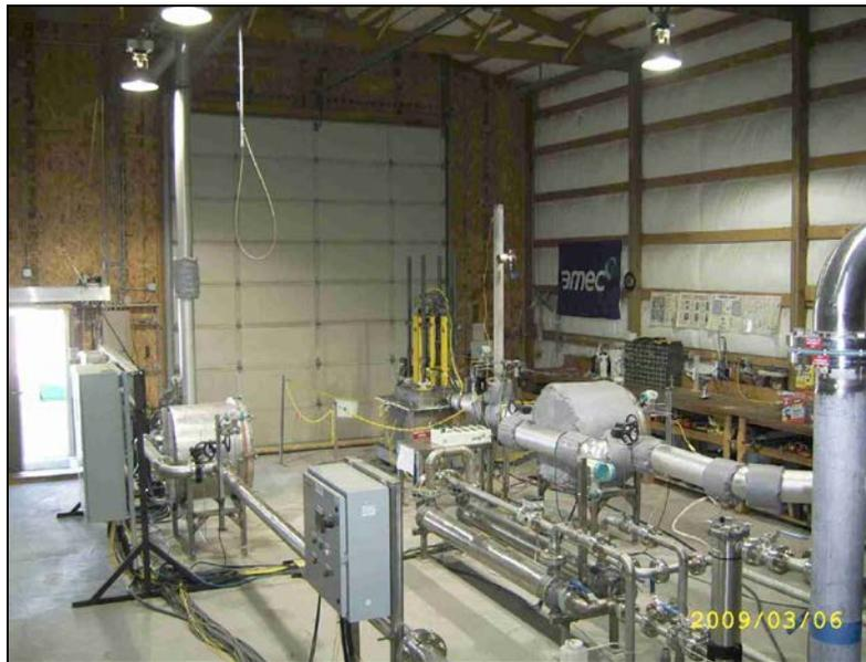
**Figure 2 - 200-liter GeoMelt® Vitrification Equipment inside the Horn Rapids Test Site**
