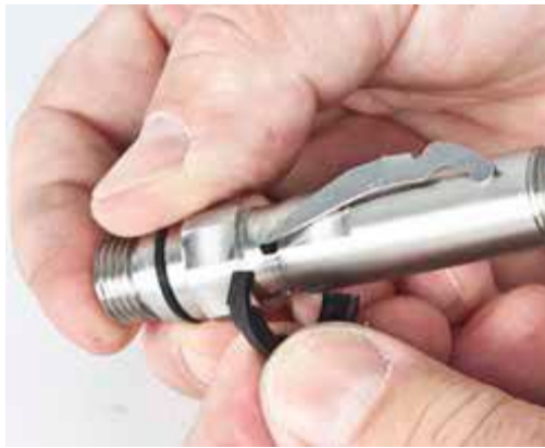
卸下摇杆臂支撑夹
