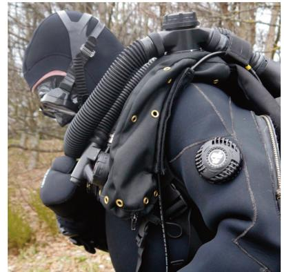
Gas is stored in a back mounted twin 2 litre cylinder assembly, which is monitored by a pressure gauge and is supplied to the breathing circuit via an adjustable Constant Mass Flow (CMF) metering valve. Additionally gas is also supplied to a demand valve that automatically provides counterlung volume during descent, whilst serving as a manual gas addition (bypass) valve.
